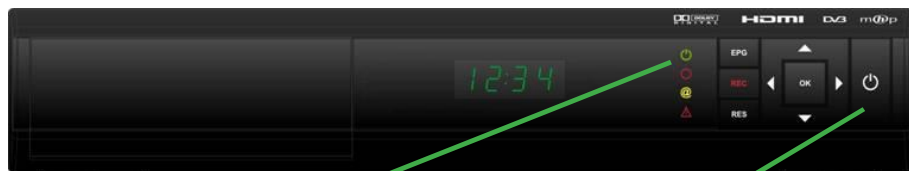
Power on indicator light (green)
